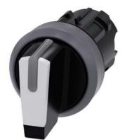
Selector switch, illuminable, 22 mm, round, plastic with metal front ring, white, selector switch, short, 3 switch positions I-O<II, left latching, right momentary contact type, actuating angle 2x45°, 10:30h/12h/13:30h, with laser labeling, inscription or symbol Customer-specific selection with SIRIUS ACT configurator (CIN)
