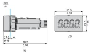
e: Clamping thickness 1 to 6 mm
