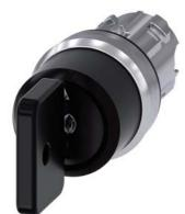
Key-operated switch O.M.R, 22 mm, round, metal, shiny, lock number 73034, black, with 2 keys, 3 switch positions I-O-II, latching, actuating angle 2x45°, 10:30h/12h/13:30h, key removal O, with laser labeling, lower case
