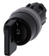
Key-operated switch O.M.R, 22 mm, round, plastic with metal front ring, lock number 73034, black, with 2 keys, 3 switch positions I-O-II, latching, actuating angle 2x45°, 10:30h/12h/13:30h, key removal O, with laser labeling, inscription or symbol Customer-specific selection with SIRIUS ACT configurator (CIN)
