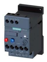
Overload relay 5.5...8.0 A Thermal For motor protection Size S00, Class 10 Stand-alone installation Main circuit: Screw Auxiliary circuit: Screw Manual-Automatic-Reset
