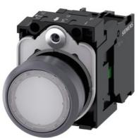
Illuminated pushbutton, 22 mm, round, plastic with metal front ring, white, pushbutton, flat, momentary contact type, with holder, 1NO, LED module with integrated LED 24 V AC/DC, screw terminal, with laser labeling, symbol number according to, ISO 7000 or IEC 60417
