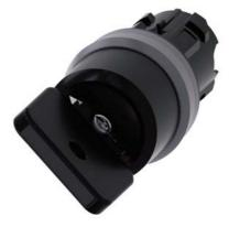
Key-operated switch O.M.R, 22 mm, round, plastic with metal front ring, lock number 73034, black, with 2 keys, 2 switch positions O-I, latching, actuating angle  $90^\circ,\,10:\!30h/13:\!30h,$  key removal I, Z=50-unit packaging
