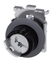
RONIS key-operated switch, 30 mm, round, Metal, matte, front ring for flush installation, lock number SB30, with 2 keys, 2 switch positions O<I, momentary contact type, Actuating angle 45°, 10:30h/12h, key removal O, possible special locks: SB31, 421, 455, Z=50-unit packaging
