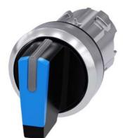
Selector switch, illuminable, 22 mm, round, metal, shiny, blue, selector switch, short, 3 switch positions I>O<II, momentary contact type, actuating angle 2x45°, 10:30h/12h/13:30h, Z=50-unit packaging
