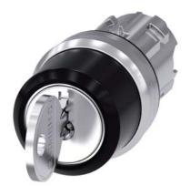
RONIS key-operated switch, 22 mm, round, metal, shiny, lock number SB30, with 2 keys, 3 switch positions I>O<II, momentary contact type, actuating angle 2x45°, 10:30h/12h/13:30h, key removal O, possible special locks: SB31, 421, 455, with laser labeling, upper case and lower case, always upper case at the beginning of the word
