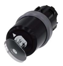
Key-operated switch BKS, 22 mm, round, plastic with metal front ring, Lock number E1 (VW), without key, 2 switch positions O-I, latching, actuating angle 90°, 10:30h/13:30h, key removal O+I, with laser labeling, upper case and lower case, always upper case at beginning of line
