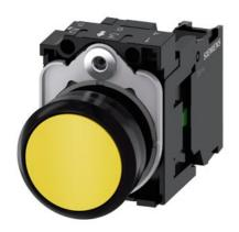
Pushbutton, 22 mm, round, plastic, yellow, pushbutton, flat, momentary contact type, with holder 1 NO, screw terminal, with laser labeling, upper case
