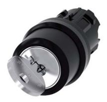
RONIS key-operated switch, 22 mm, round, plastic, lock number SB30, with 2 keys, 2 switch positions O<I, momentary contact type, Actuating angle 45°, 10:30h/12h, key removal O, possible special locks: SB31, 421, 455, with laser labeling, upper case and lower case, always upper case at the beginning of the word
