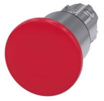
Mushroom pushbutton, 22 mm, round, metal, shiny, red, 40 mm, 3 switch positions, latches after pushing in, unlatches by pull-to-unlatch mechanism to center position, after pulling out the button Retraction to center position, with laser labeling, symbol number according to, ISO 7000 or IEC 60417
