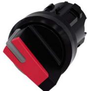
Selector switch, illuminable, 22 mm, round, plastic, red, selector switch, short, 2 switch positions O-I, latching, actuating angle 90°, 10:30h/13:30h Z=50-unit packaging
