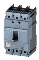
circuit breaker 3VA5 UL frame 125 breaking capacity class H 65kA @ 480 V 3-pole, line protection TM230, FTAM, In=30A overload protection Ir=30A fixed short-circuit protection Ii=5...10 x In UL489 SB (naval), 50 deg. cel. cable connection on both sides
