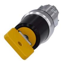
Key-operated switch O.M.R, 22 mm, round, metal, shiny, lock number 73033, yellow, with 2 keys, 2 switch positions O-I, latching, actuating angle 90°, 10:30h/13:30h, key removal O+I, with laser labeling, upper case
