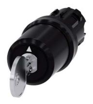
Key-operated switch BKS, 22 mm, round, plastic, Lock No. E9 (VW), without key, 3 switch positions I-O-II, latching, actuating angle 2x45°, 10:30h/12h/13:30h, Key removal I+O+II, with laser labeling, upper case and lower case, always upper case at beginning of line
