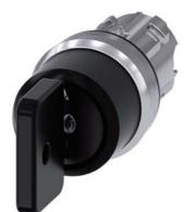
Key-operated switch O.M.R, 22 mm, round, metal, shiny, lock number 73034, black, with 2 keys, 3 switch positions I-O-II, latching, actuating angle 2x45°, 10:30h/12h/13:30h, key removal O, with laser labeling, upper case
