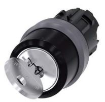
RONIS key-operated switch, 22 mm, round, plastic with metal front ring, lock number SB30, with 2 keys, 2 switch positions O-I, latching, actuating angle 90°, 10:30h/13:30h, key removal O+I, possible special locks: SB31, 421, 455, with laser labeling, upper case and lower case, always upper case at the beginning of the word
