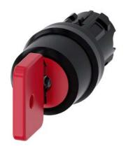
Key-operated switch O.M.R, 22 mm, round, plastic, lock number 73037, red, with 2 keys, 3 switch positions I-O-II, latching, actuating angle 2x45°, 10:30h/12h/13:30h, key removal O, with laser labeling, inscription or symbol Customer-specific selection with SIRIUS ACT configurator (CIN)
