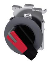
Selector switch, illuminable, 30 mm, round, Metal, matte, red, selector switch, long, front ring for flush installation, 2 switch positions O<I, momentary contact type, Actuating angle 45°, 10:30h/12h, with laser labeling, upper case and lower case, always upper case at the beginning of the word
