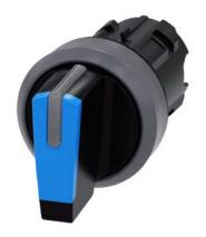
Selector switch, illuminable, 22 mm, round, plastic with metal front ring, blue, selector switch, short, 3 switch positions I>O<II, momentary contact type, actuating angle 2x45°, 10:30h/12h/13:30h, with laser labeling, lower case
