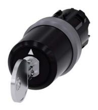
Key-operated switch BKS, 22 mm, round, plastic with metal front ring, lock number S1, with 2 keys, 3 switch positions I-O-II, latching, actuating angle 2x45°, 10:30h/12h/13:30h, Key removal II, with laser labeling, inscription or symbol Customer-specific selection with SIRIUS ACT configurator (CIN)
