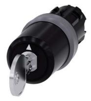
Key-operated switch BKS, 22 mm, round, plastic with metal front ring, Lock No. E2 (VW), without key, 3 switch positions I-O-II, latching, actuating angle 2x45°, 10:30h/12h/13:30h, Key removal I+O+II, Z=50-unit packaging
