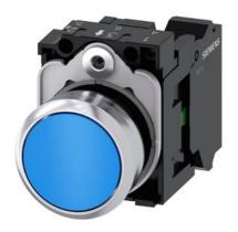
Pushbutton, 22 mm, round, metal, shiny, blue, pushbutton, flat, momentary contact type, 1 NO, spring-type terminal, with laser labeling, inscription or symbol Customer-specific selection with SIRIUS ACT configurator (CIN)
