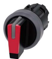
Selector switch, illuminable, 22 mm, round, plastic with metal front ring, red, selector switch, short, 3 switch positions I>O<II, momentary contact on the left, latching on the right, actuating angle 2x45°, 10:30h/12h/13:30h, with laser labeling, inscription or symbol Customer-specific selection with SIRIUS ACT configurator (CIN)
