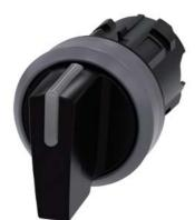
Illuminable selector switch, 22 mm, round, plastic with metal front ring, black, Selector switch short, 3 switch positions I-O<II, left latching, right momentary contact type, actuating angle 2x45°, 10:30h/12h/13:30h
