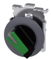
Selector switch, illuminable, 30 mm, round, Metal, matte, green, selector switch, short, front ring for flush installation, 2 switch positions O-I, latching, actuating angle 90°, 10:30h/13:30h, with laser labeling, inscription or symbol Customer-specific selection with SIRIUS ACT configurator (CIN)
