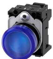
Indicator lights, 22 mm, round, metal, shiny, blue, lens, smooth, with holder, LED module with integrated LED 24 V AC/DC, spring-type terminal, with laser labeling, symbol number according to, ISO 7000 or IEC 60417
