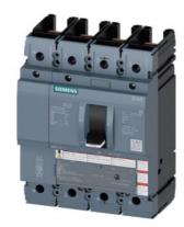
circuit breaker 3VA5 UL frame 250 breaking capacity class H 65kA @ 480V 4-pole, line protection TM210, FTFM, In=90A overload protection Ir=90A fixed short-circuit protection Ii=10 x In N conductor unprotected without connection
