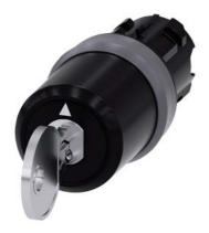
key-operated switch Siemens, 22 mm, round, plastic with metal front ring, lock number SSG10, with 2 keys, 3 switch positions I-O<II, left latching, momentary contact type on the right, actuating angle 2x45°, 10:30h/12h/13:30h, key removal O, with laser labeling, inscription or symbol customer-specific selection with SIRIUS ACT configurator (CIN)
