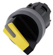
Selector switch, illuminable, 22 mm, round, plastic with metal front ring, yellow, selector switch, short, 2 switch positions O-I, latching, actuating angle 90°, 10:30h/13:30h, with laser labeling, upper case
