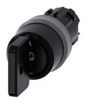
Key-operated switch O.M.R, 22 mm, round, plastic with metal front ring, lock number 73034, black, with 2 keys, 3 switch positions I-O-II, latching, actuating angle 2x45°, 10:30h/12h/13:30h, key removal O, with laser labeling, upper case and lower case, always upper case at the beginning of the word
