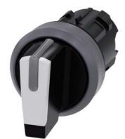
Selector switch, illuminable, 22 mm, round, plastic with metal front ring, white, selector switch, short, 3 switch positions I-O<II, left latching, right momentary contact type, actuating angle 2x45°, 10:30h/12h/13:30h, Z=50-unit packaging
