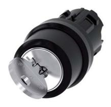
RONIS key-operated switch, 22 mm, round, plastic, lock number 455, with 2 keys, 2 switch positions O-I, latching, actuating angle  $90^\circ$ , 10:30h/13:30h, key removal O+I, with laser labeling, lower case
