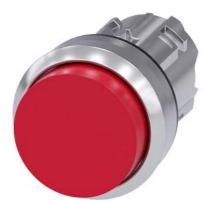
Pushbutton, 22 mm, round, metal, shiny, red, pushbutton, high, latching, Push-to-release mechanism, with laser labeling, upper case and lower case, always upper case at the beginning of the word
