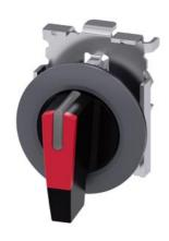
Selector switch, illuminable, 30 mm, round, Metal, matte, red, selector switch, long, front ring for flush installation, 3 switch positions I-O-II, latching, actuating angle 2x45°, 10:30h/12h/13:30h, with laser labeling, lower case
