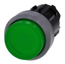
Illuminated pushbutton, 22 mm, round, plastic with metal front ring, green, pushbutton, raised momentary contact type, with laser labeling, symbol number according to, ISO 7000 or IEC 60417
