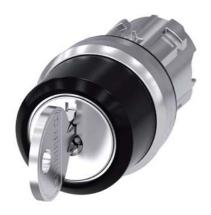
RONIS key-operated switch, 22 mm, round, metal, shiny, lock number SB30, with 2 keys, 3 switch positions I-O<II, left latching, right momentary contact type, actuating angle 2x45°, 10:30h/12h/13:30h, key removal O+I, possible special locks: SB31, 421, 455, Z=50-unit packaging
