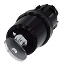
key-operated switch Siemens, 22 mm, round, plastic, lock no. LSG1, with 2 keys, 2 switch positions O<I, momentary contact type, actuating angle  $45^\circ,\,10:30h/12h,$  key removal O, with laser labeling, upper case and lower case, always upper case at beginning of line
