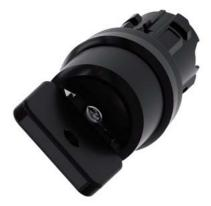
Key-operated switch O.M.R, 22 mm, round, plastic, lock number 73034, black, with 2 keys, 2 switch positions O-I, latching, actuating angle 90°, 10:30h/13:30h, Key removal I Z=50-unit packaging
