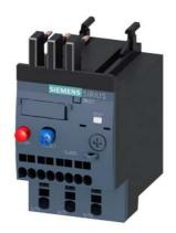
Overload relay 0.22...0.32 A Thermal For motor protection Size S00, Class 10 Contactor mounting Main circuit: Spring-type terminal Auxiliary circuit: spring-type terminal Manual-Automatic-Reset
