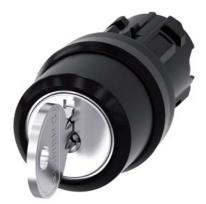
RONIS key-operated switch, 22 mm, round, plastic, lock number SB30, with 2 keys, 3 switch positions I-O-II, latching, actuating angle 2x45°, 10:30h/12h/13:30h, Key removal I+O+II, possible special locks: SB31, 421, 455, with laser labeling, upper case and lower case, always upper case at the beginning of the word
