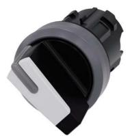
Selector switch, illuminable, 22 mm, round, plastic with metal front ring, white, selector switch, short, 2 switch positions O<I, momentary contact type, Actuating angle 45°, 10:30h/12h, with laser labeling, upper case and lower case, always upper case at beginning of line
