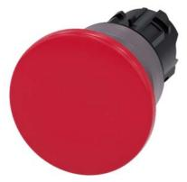
Mushroom pushbutton, 22 mm, round, plastic with metal front ring, red, 40mm, momentary contact type, with laser labeling, upper case
