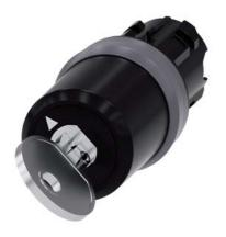
key-operated switch Siemens, 22 mm, round, plastic with metal front ring, lock number SSG10, with 2 keys, 2 switch positions O-I, latching, actuating angle 90°, 10:30h/13:30h, key removal O, with laser labeling, upper case and lower case, always upper case at beginning of line
