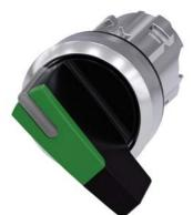
Selector switch, illuminable, 22 mm, round, metal, shiny, green, selector switch, long, 2 switch positions O<I, momentary contact type, Actuating angle 45°, 10:30h/12h, Z=50-unit packaging
