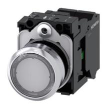
Illuminated pushbutton, 22 mm, round, metal, shiny, clear, pushbutton, flat, momentary contact type, with holder, 1NO, LED module with integrated LED 110 V AC, spring-type terminal, Z=20-unit packaging
