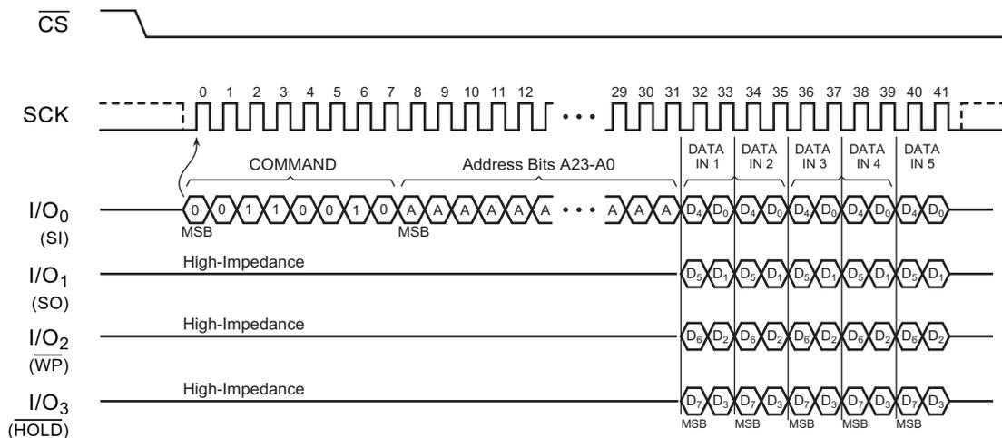
Figure 32. Quad Page Program Sequence Diagram
