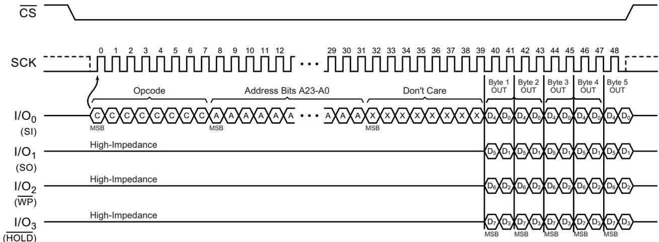
Figure 11. Quad Output Fast Read Sequence Diagram
