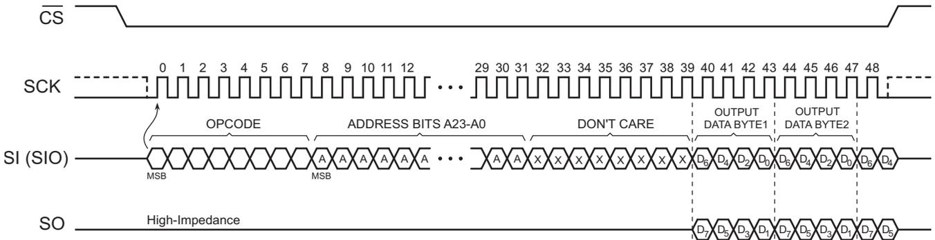
Figure 10. Dual Output Fast Read Sequence Diagram
