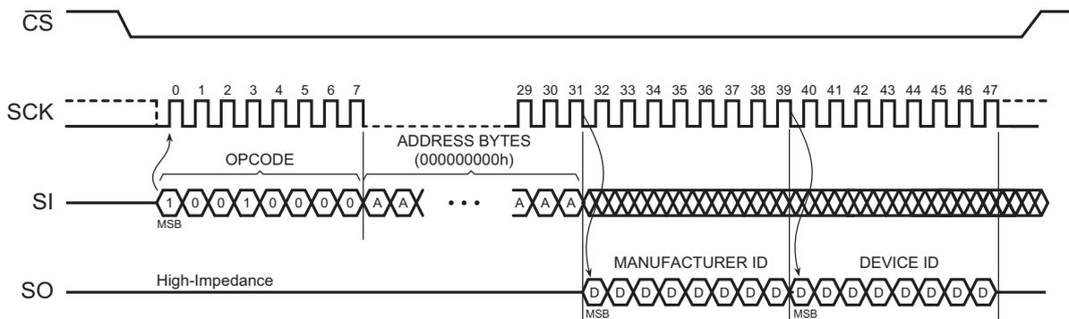
Figure 19. Read Manufacturer ID/ Device ID Sequence Diagram
