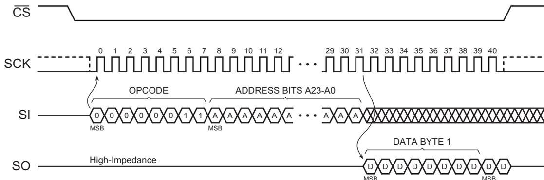
Figure 8. Read Data Bytes Sequence Diagram
