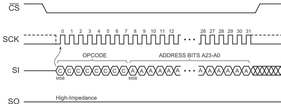
Figure 35. 32 kbytes Block Erase Sequence Diagram
