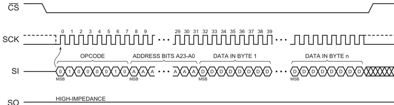
Figure 29. Program Security Registers Command Sequence Diagram
