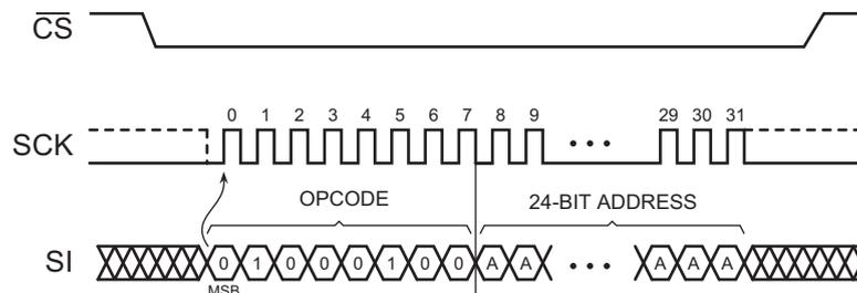
Figure 28. Erase Security Registers Command Sequence Diagram
