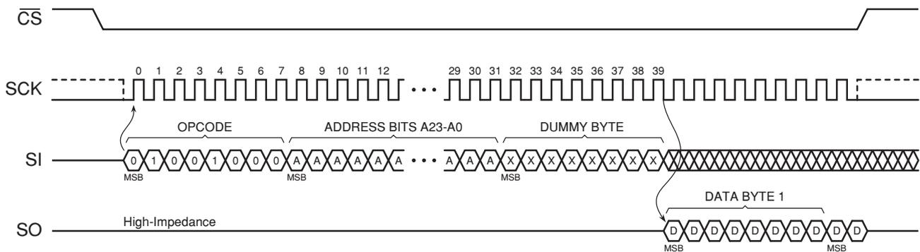
Figure 27. Read Security Registers Command Sequence Diagram
