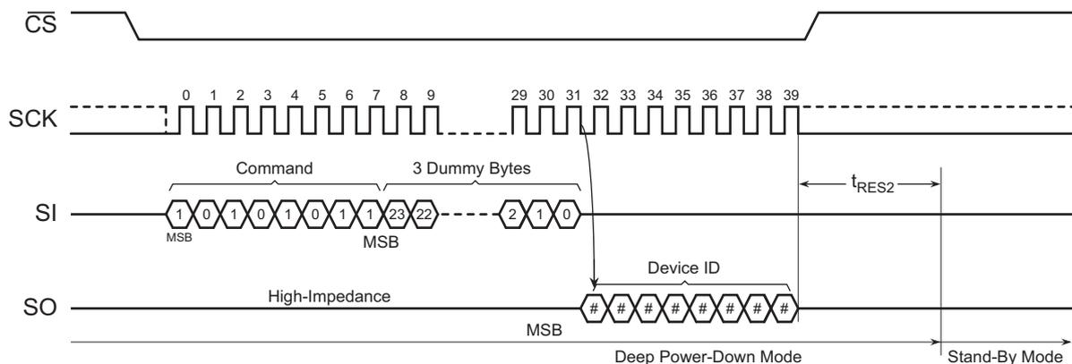
Figure 26. Release Power-Down/Read Device ID Sequence Diagram
