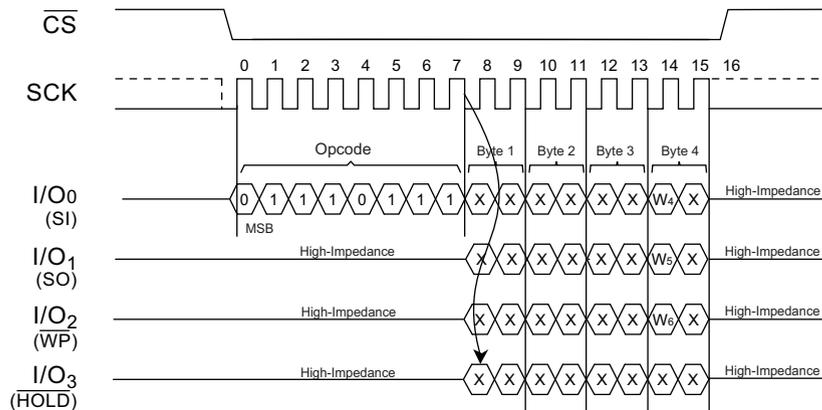
Figure 18. Set Burst with Wrap Sequence Diagram
