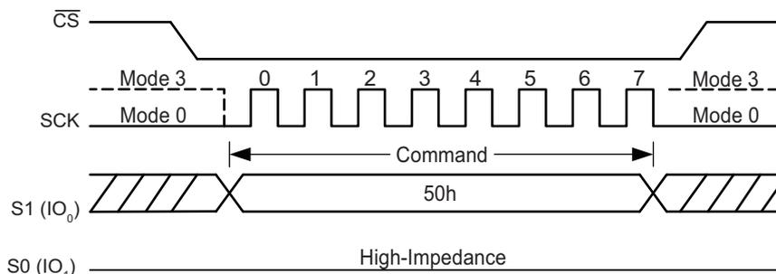
Figure 7. Write Enable for Volatile Status Register
