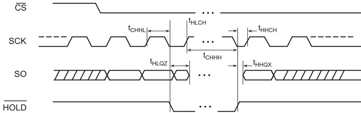
Figure 45.  $\overline{HOLD}$  Timing
