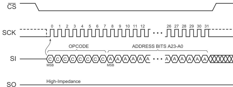
Figure 36. 64 kbytes Block Erase Sequence Diagram
