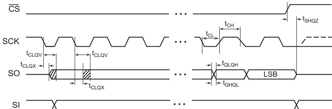
Figure 44. Output Timing
